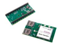
Easily integrated into any new or existing hardware applications via its standard 49-pin DIP configuration, the LTE910CF is a cost-effective solution for LTE IoT (Internet of Things) connectivity. Users can choose to mount the devices directly onto their PC Board or simply mount in a DIP socket or header. Their footprint compatibility with other Janus products removes the worry of obsolescence.
